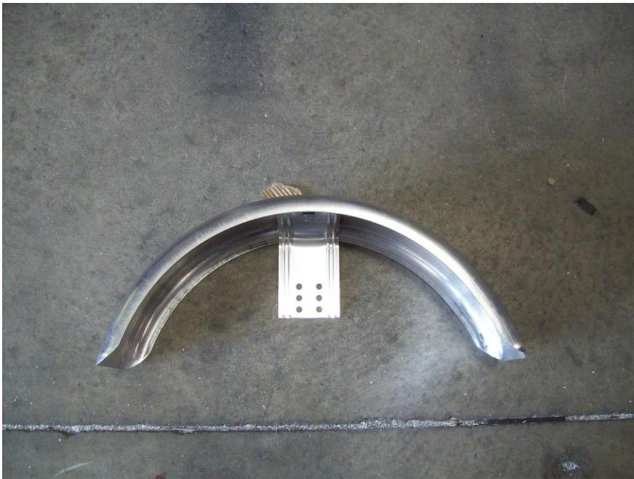
Locate the fender with mounting bracket.
