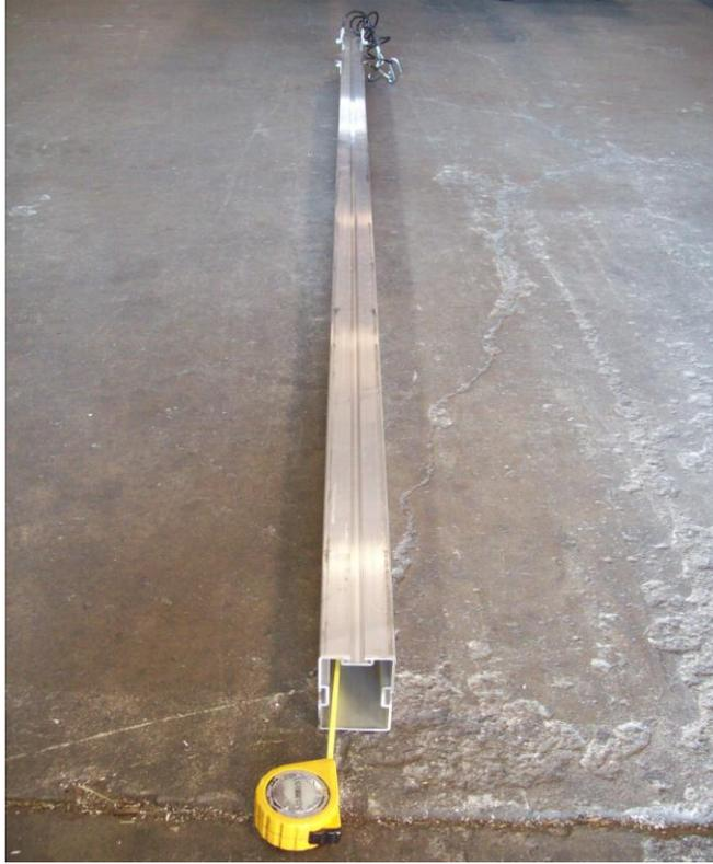
Extend a tape measure inside the tongue from the rear of the trailer until it protrudes at the front of the trailer under the coupler.
