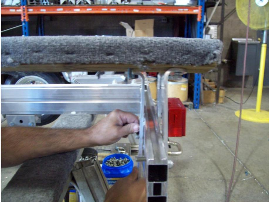
After you install the outside bunk boards go back and add the slotted angle brackets to front of each board as shown. Final adjustment will be made when boat is on the trailer.
