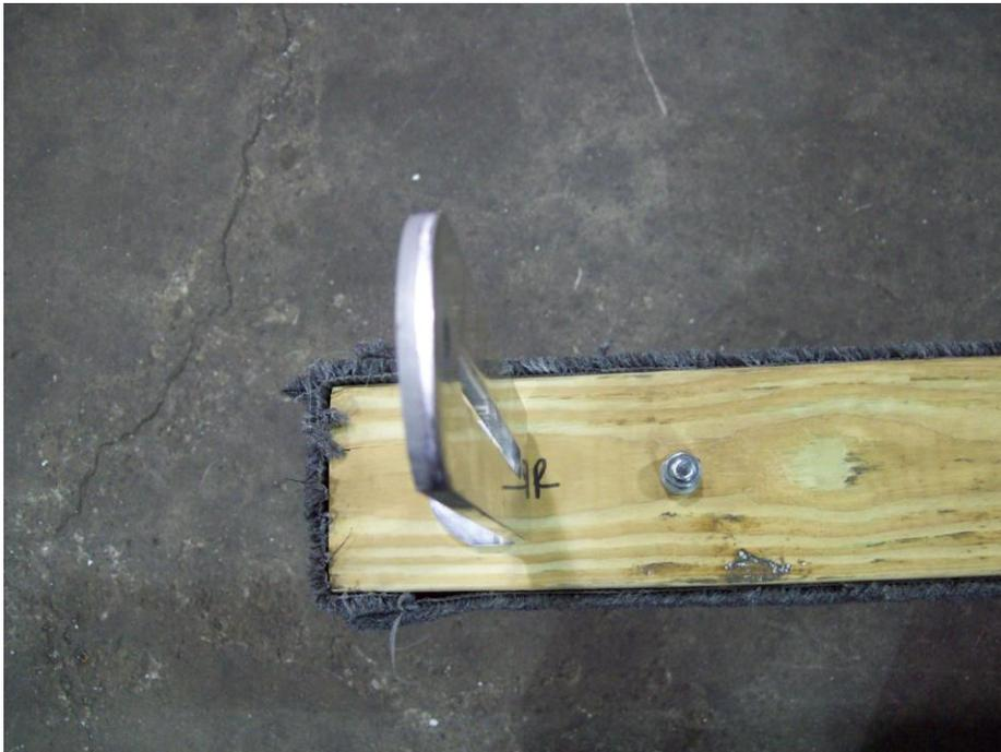
Install the slotted angle brackets to the front and rear of the bunk boards as shown.
