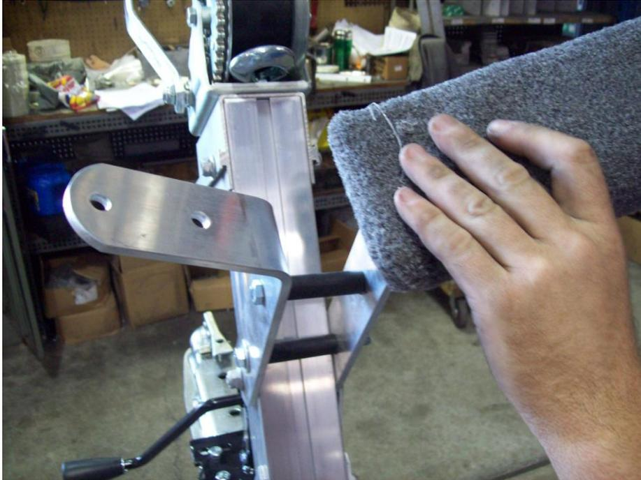
Install the bunk boards to the angle brackets of the winch post.
