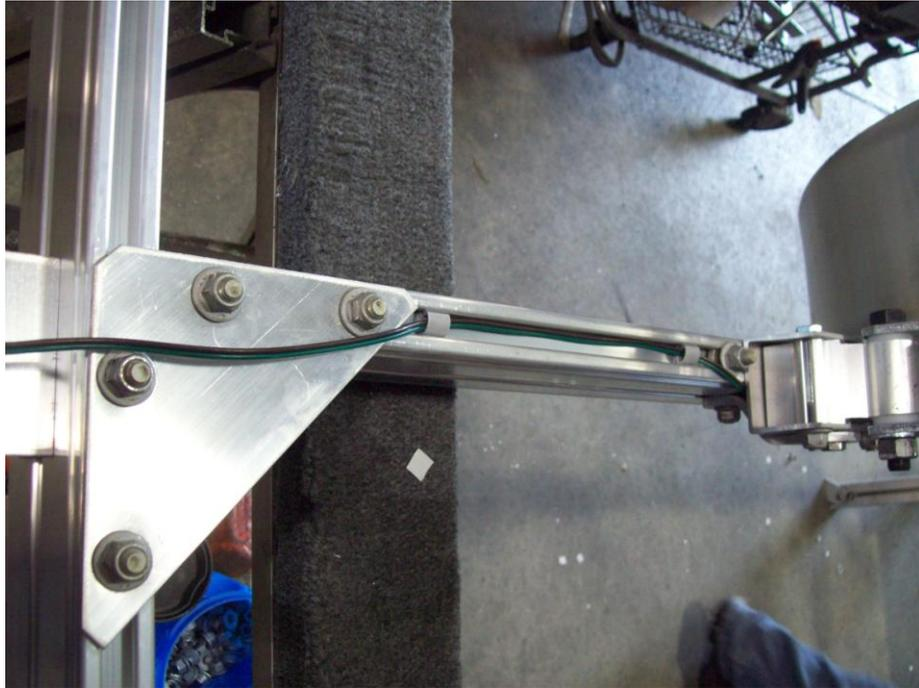
After wire is run through the channels go back and add adhesive clips to take up the slack on the harness as shown.
