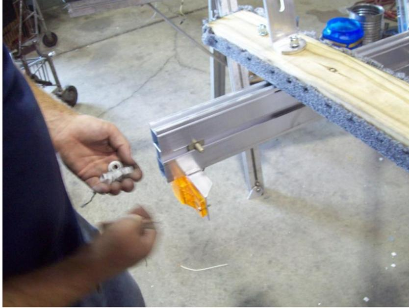
Slide one T-bolt on each side of the front and rear crossbar to mount the angle brackets.
