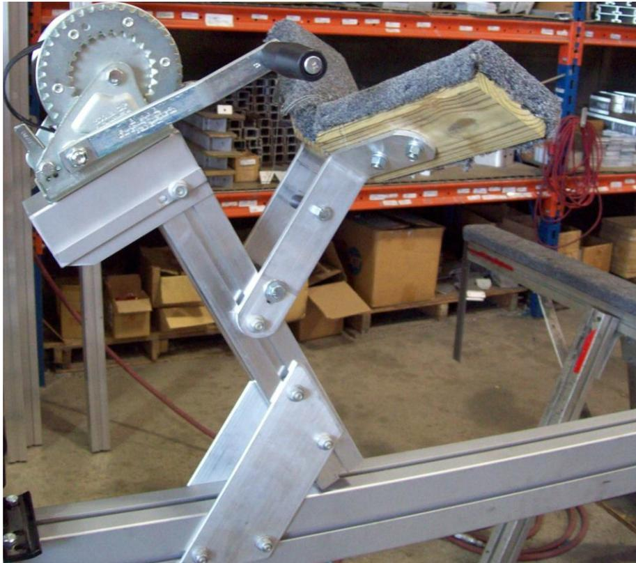
Now install winch post onto angle braces as shown. Once final placement has been determined tighten nuts on angle braces.
