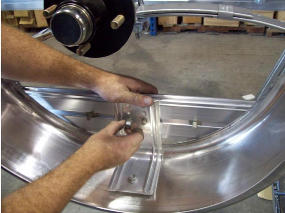
Position the four T-bolts on the side rail under the axle as shown. Install the fender bracket over the two inner T-bolts. Then position and tighten nuts.
