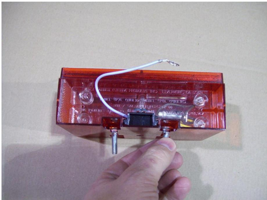
Install carriage bolts into the back of the tail lights as shown.
