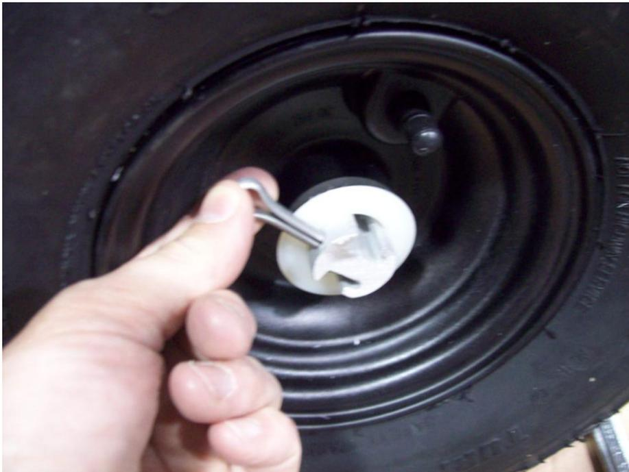
Insert cotter pin through hole on the axle.
