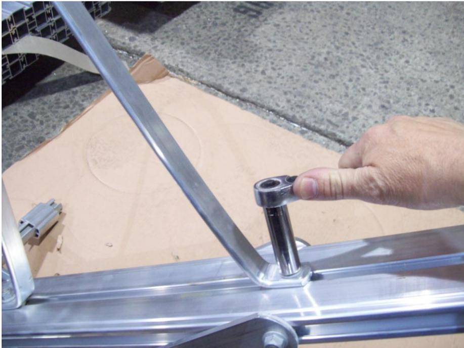
Position the back of the skid with the tongue struts as shown.
