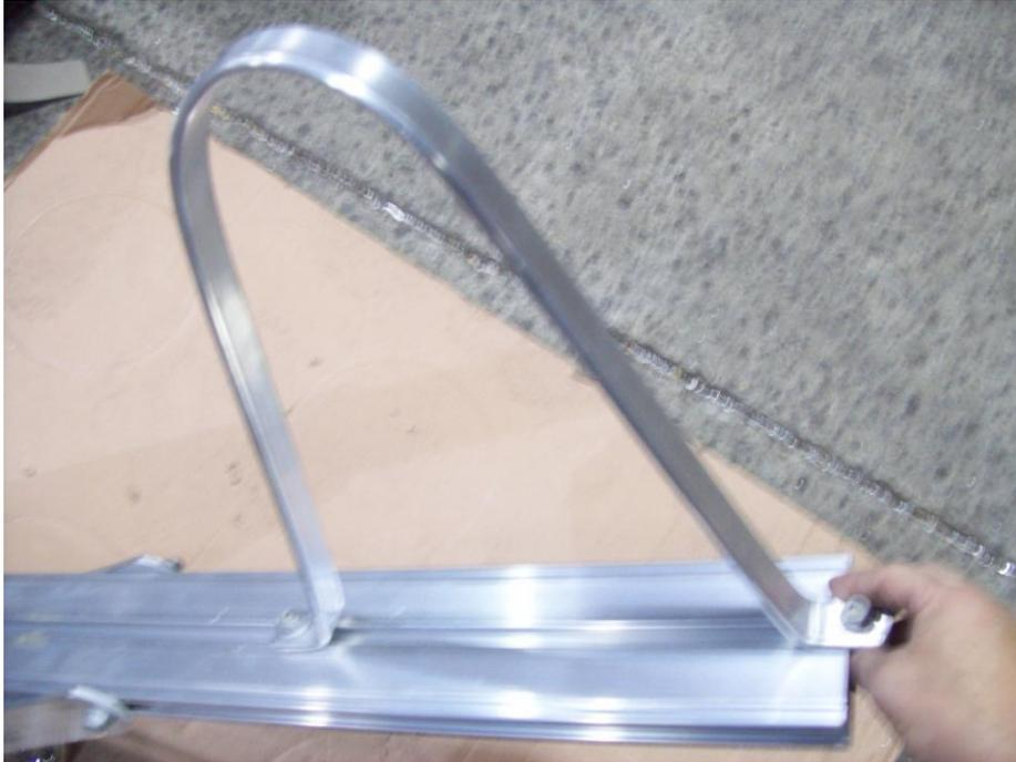
Insert the skid on the underside of the tongue as shown.
