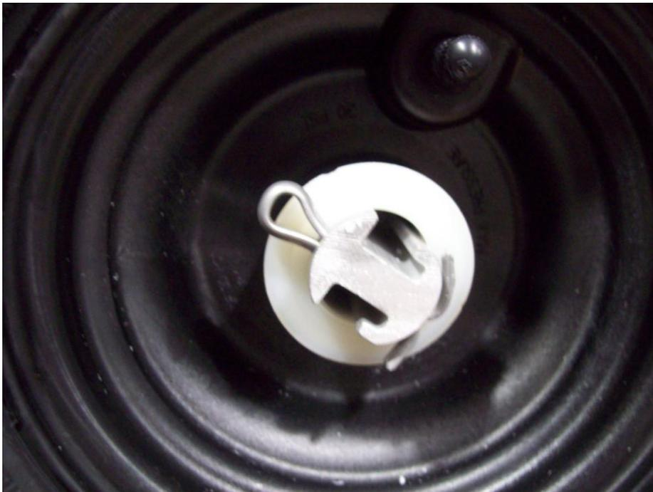
Bend the ends of the cotter pin up with a pair of pliers as shown. Then repeat this process for the other side.
