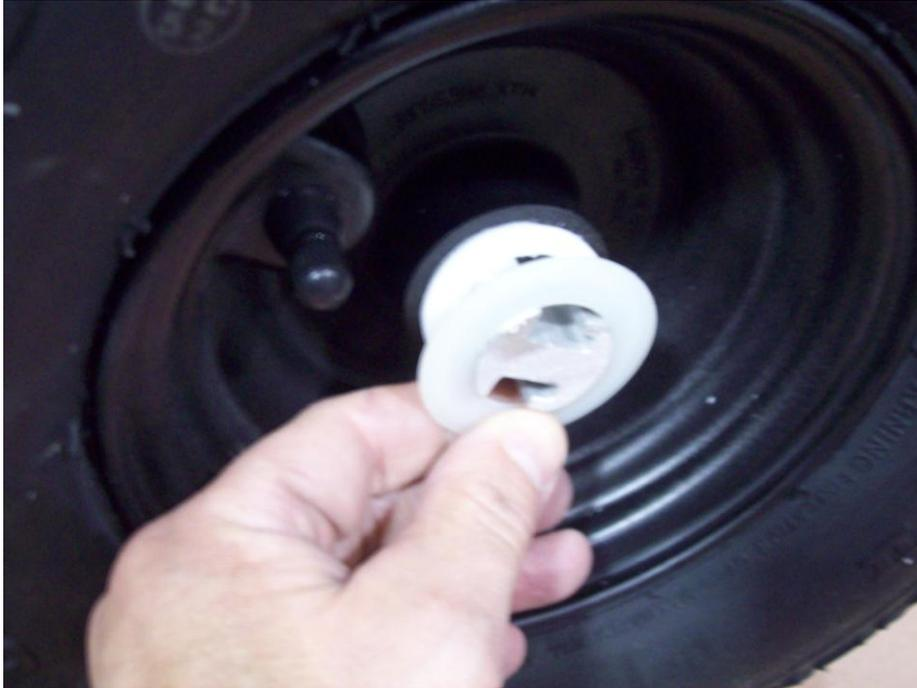
Install the tire on axle then insert the grooved side of bushing facing inward.
