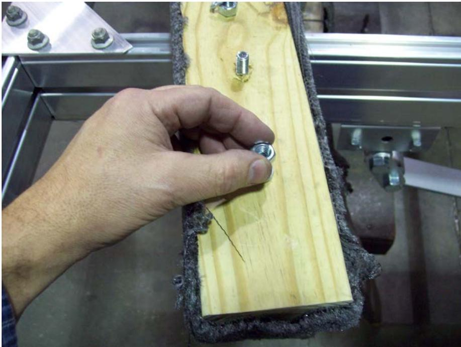
Locate the 6' padded cradles and remove nuts and lock washers.
