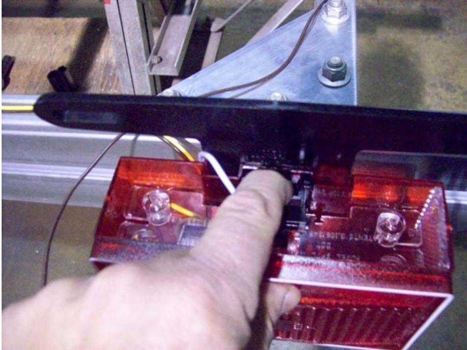
Pull black tab on the underside of the light towards the back of the trailer and up. This will release the internal portion of the light assembly.
