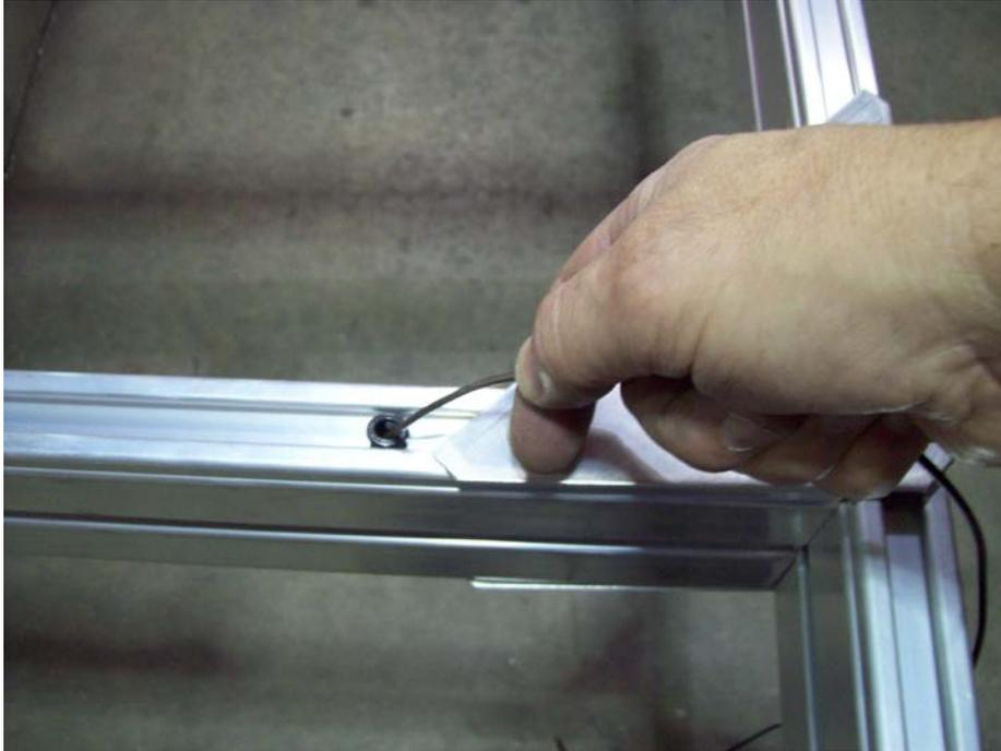
Run the wire from the clearance light down the cross arm to the side rail. Insert the wire into hole in the side rail and push wire towards the rear hole.
