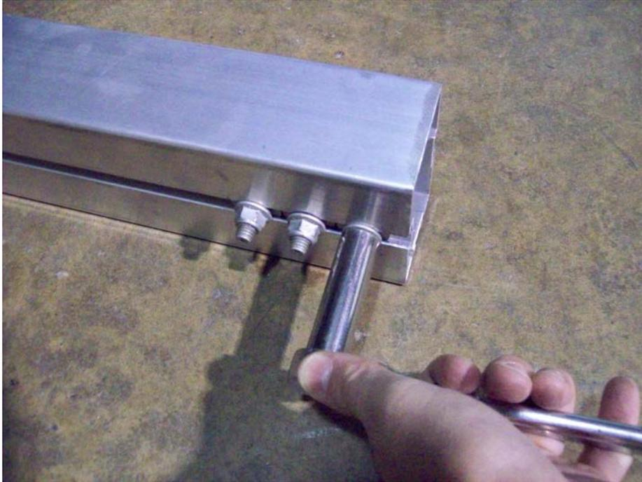
Loosen nuts on both sides of the front tongue section and slide them forward. These will be used later in the assembly process. There should be three on each side.
