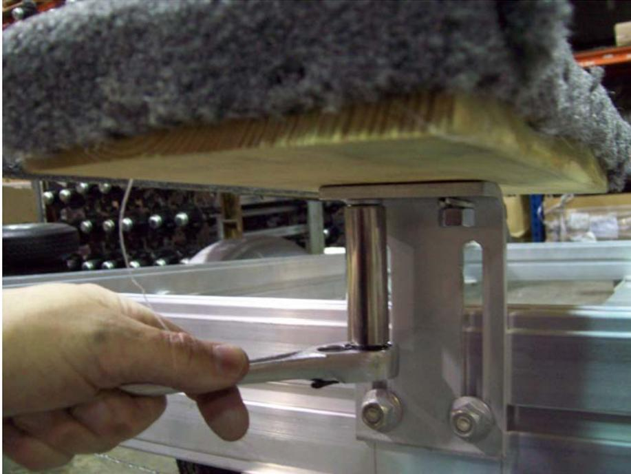
Install transom board on slotted bracket, reinstall hardware and tighten nuts.
