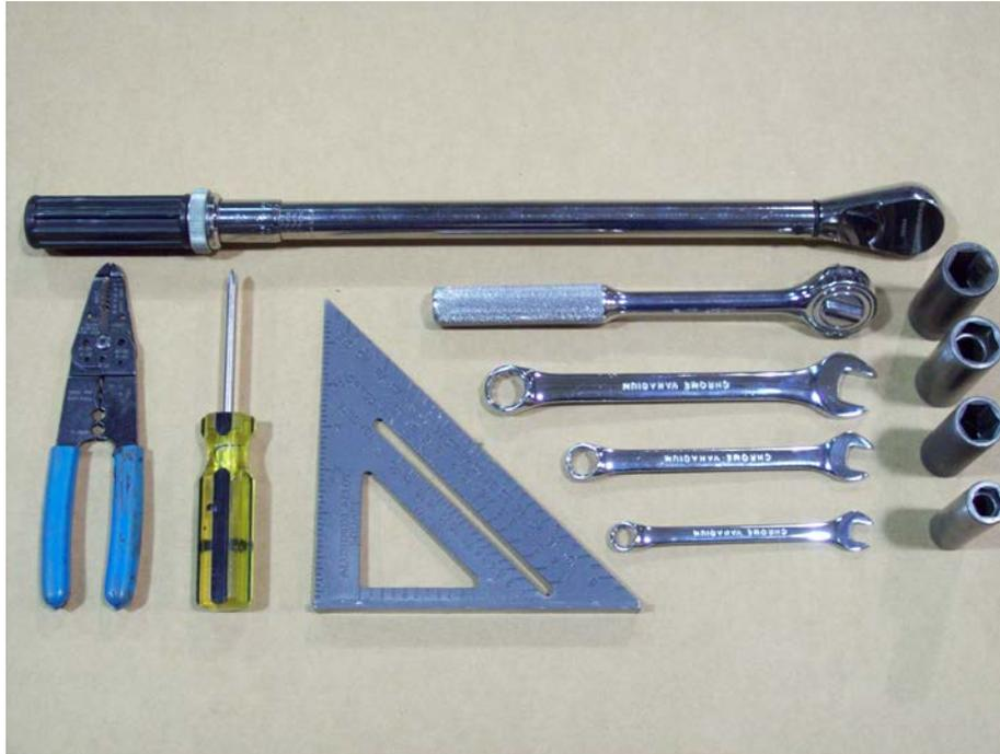
Torque wrench, carpenters square, wire cutters, Phillips screwdriver, 7/16, 9/16, and 3/4" combination wrenches, ratchet, 9/16, 3/4, 13/16", and 7/8" sockets.
