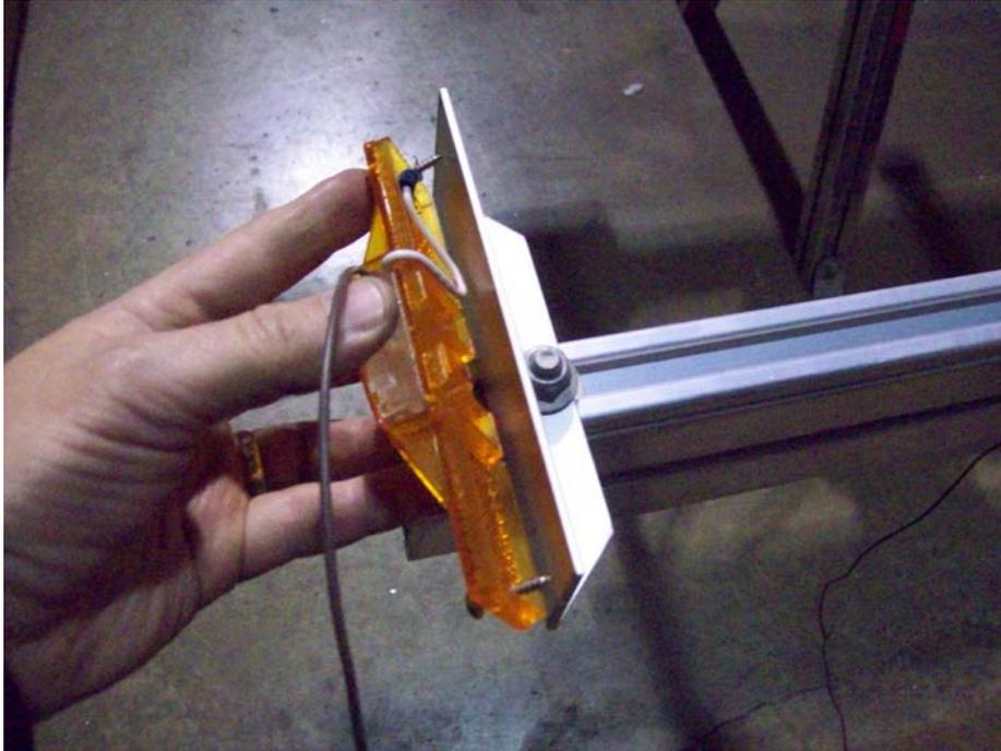
Align the ring terminal with the screw hole nearest the wire on the back of the running light. Make sure the wire is routed through the gap on the back of the light so it does not become pinched when the light is installed.
