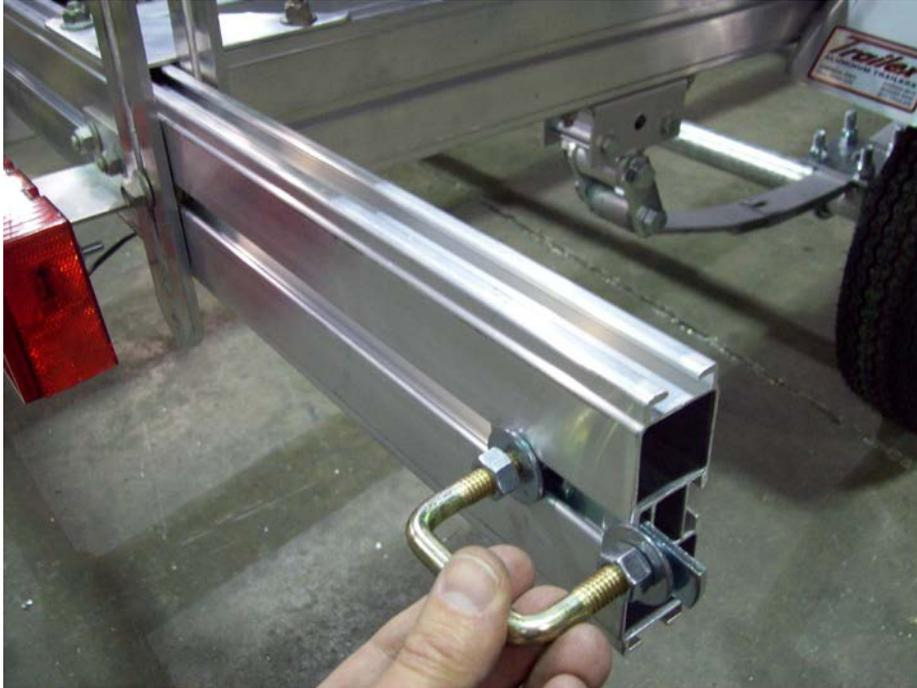
Insert web strap clips on each side of the rear cross arm.
