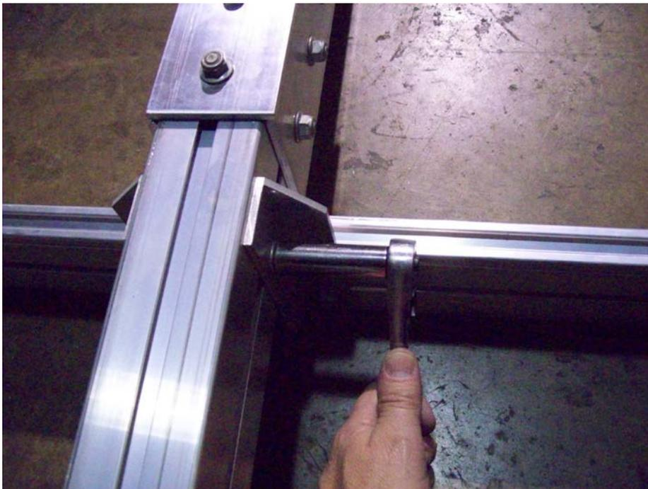
Loosen the other angle bracket, slide over and install on tongue section. Square up and tighten nuts.
