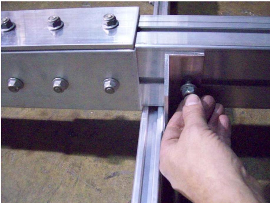
Remove the rearmost nut in the front tongue section and insert the T-bolt into the angle bracket. Reinstall nut and tighten.
