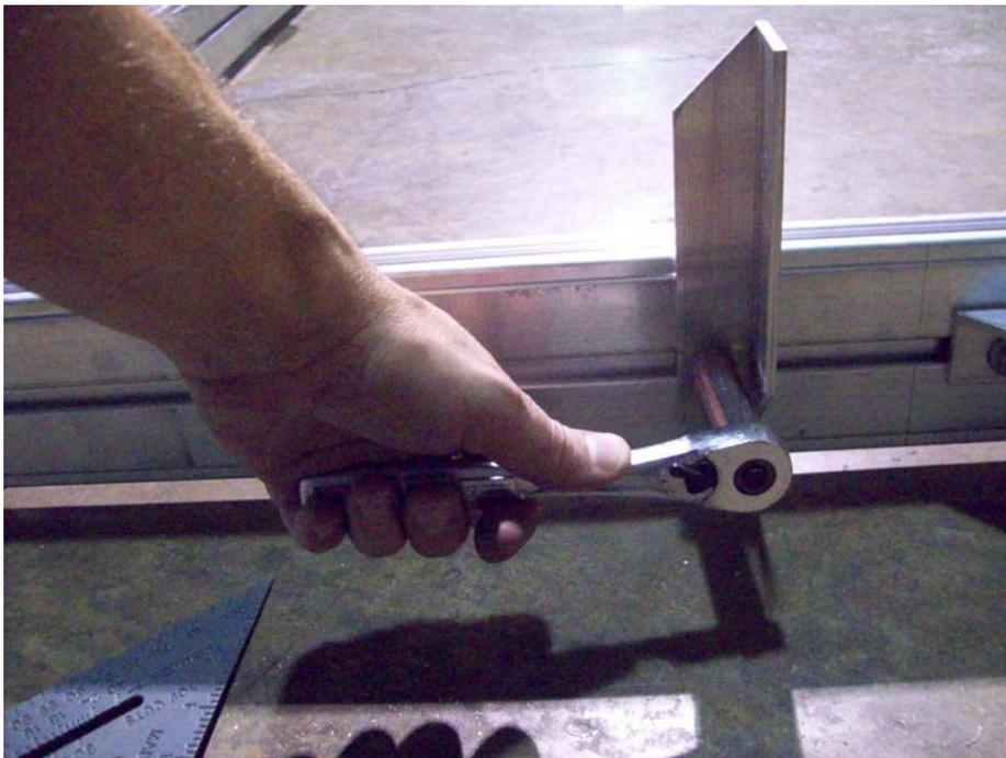
Align back edge of angle with pencil mark on cross arm. Square up angle and tighten. Leave the other angle down at this point.
