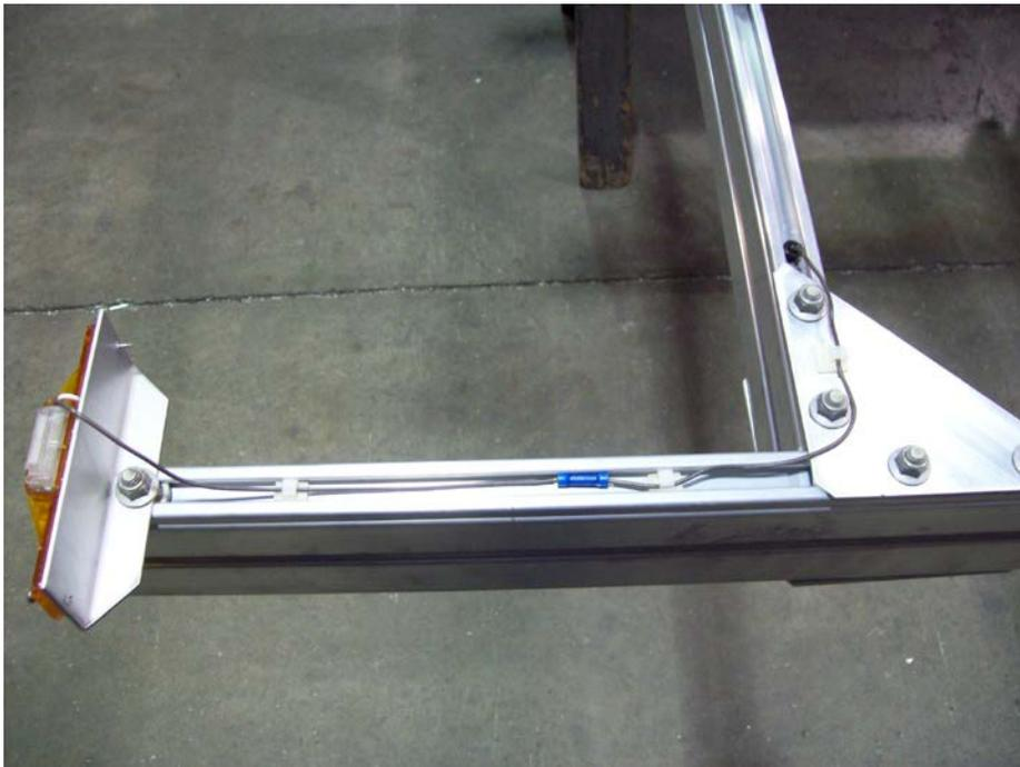
Insert adhesive clips into the cross arm and run harness through them as shown.
