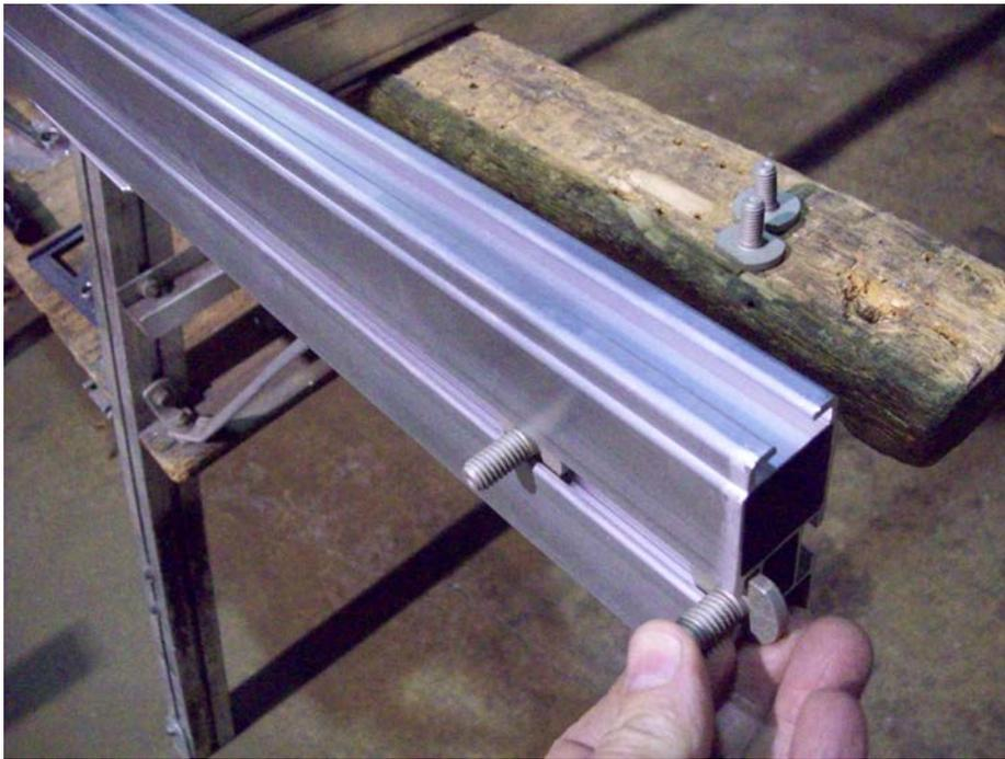
Install two T-bolts on each side of the back side of the rear cross arm.
