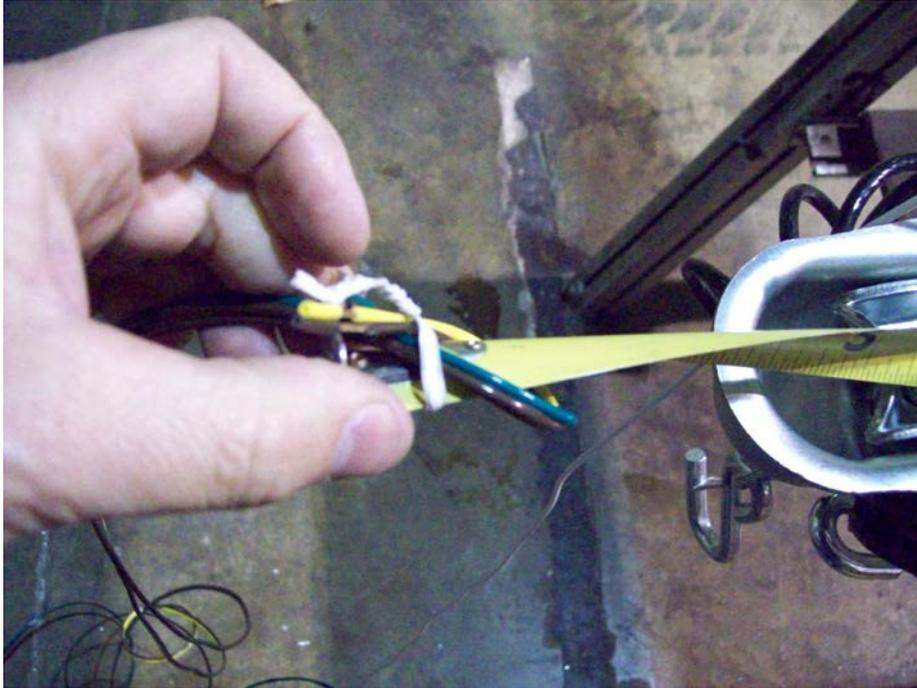
Attach both wires of the harness to the end of the tape measure with either tape or a tie.
