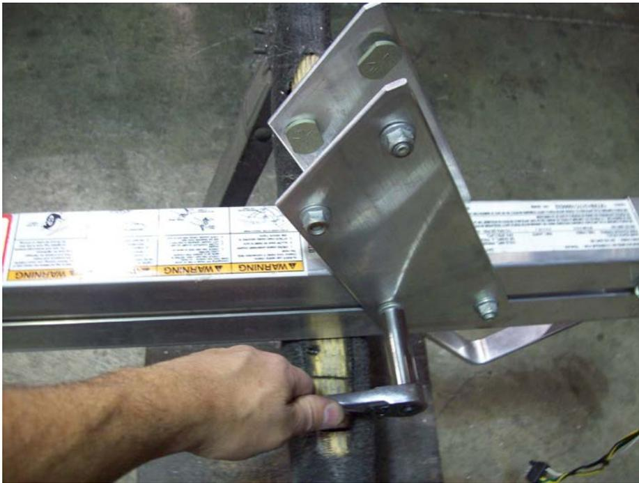
Install winch post diagonal braces on each side of the tongue section. Reinstall nuts and tighten. Final positioning will be made later to accommodate your boat.
