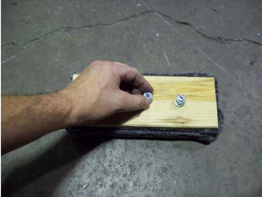
Remove the nuts and lock washers from the bow stop.
