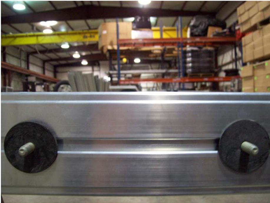
Return the trailer right side up. Slide the 1 1/8" T-bolts installed previously on page 9 into position over the axle and install two rubber washers as shown.
