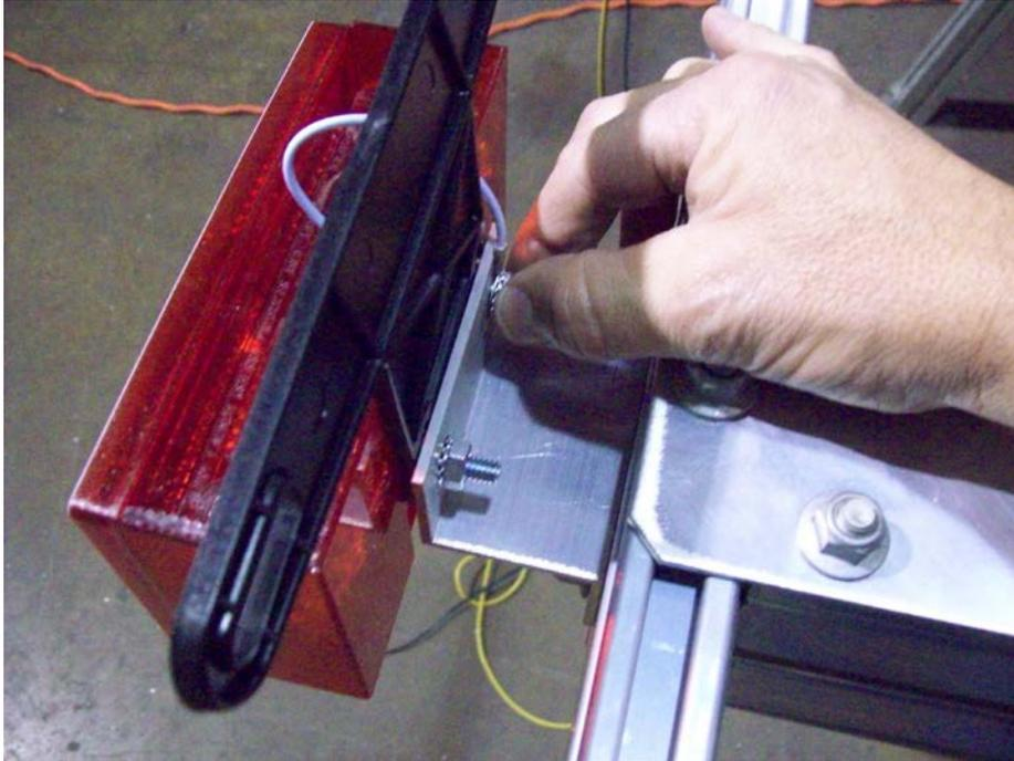
Install the left tail light with the license plate holder between the light and the bracket. Repeat for the other side. Make sure to tighten nuts but don't over tighten them. (Pictured from the bottom)
