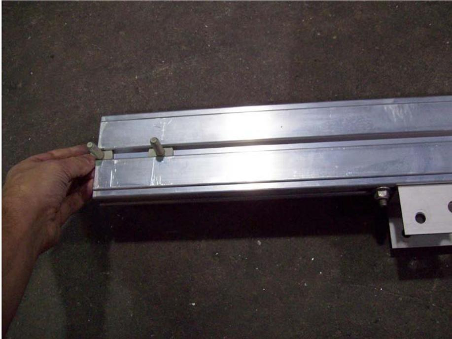
On the outward part of the side rail insert two 1 1/8" T-bolts. These will be used later to install the fenders.
