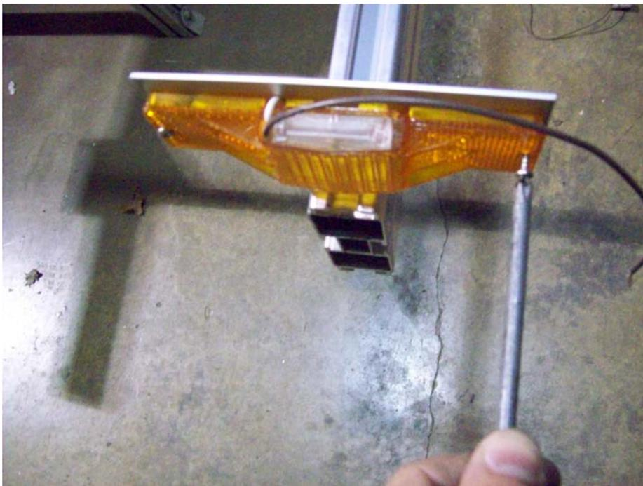
Install the running lights into the pre-drilled holes in the bracket using a Philips screwdriver. Be sure the screw is through the ring terminal on the back side of the lights. This will supply a ground to the lights. DO NOT OVER TIGHTEN.
