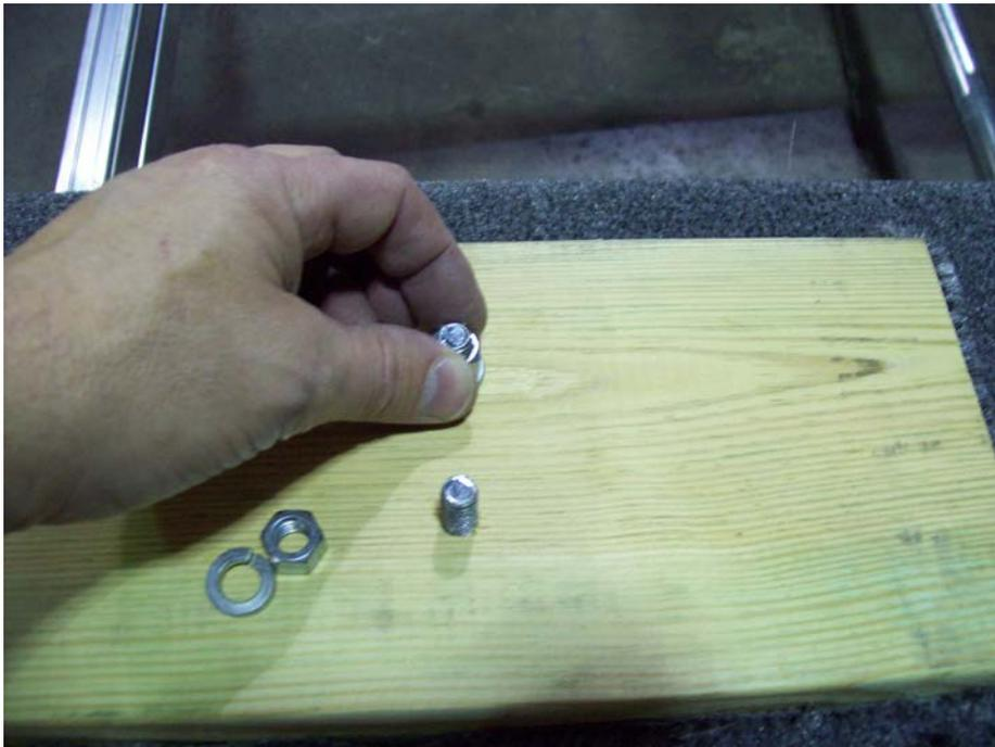
Locate the transom board and remove nuts and lock washers.
