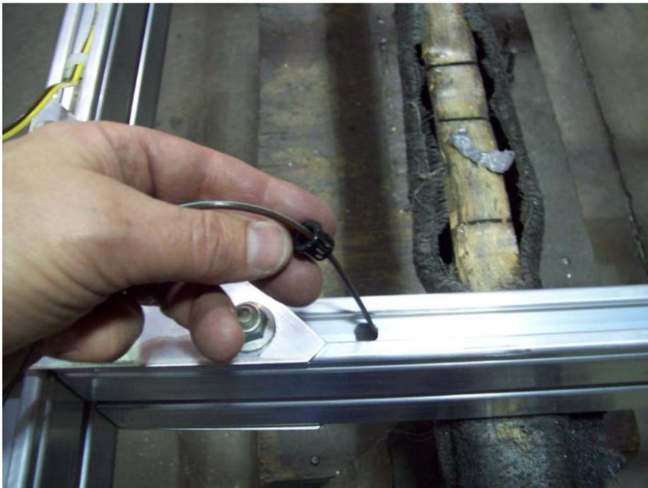
Insert wire through snap bushing and push into hole.
