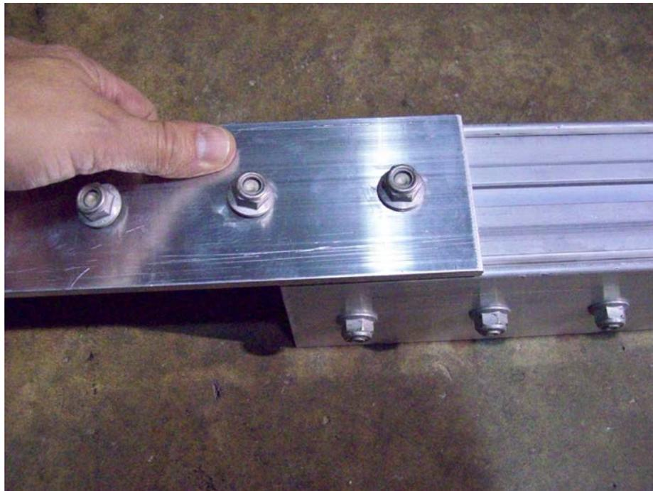
Insert splice plate into the underside of rear tongue section as shown.
