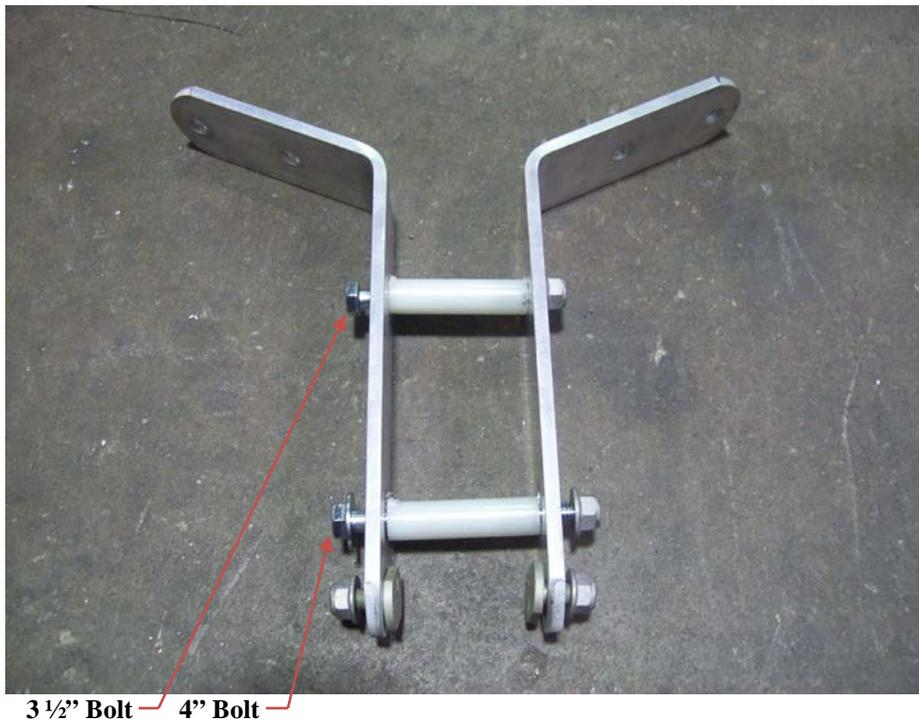
Insert the 4" bolt, flat washer, plastic sleeve, and nut in the bottom of the bow mounting brackets. Install the 3 1/2" bolt, plastic sleeve, and nut in the top hole of the bracket as shown.
