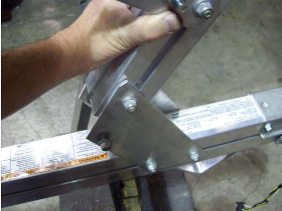
Insert winch post assembly into the T-bolts in the diagonal braces as shown.
