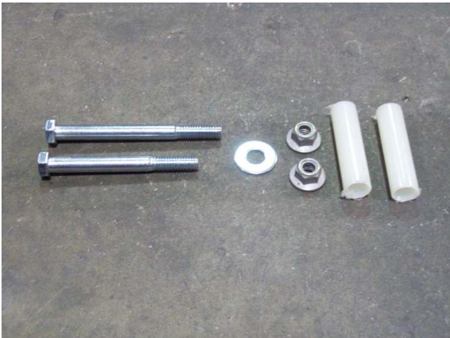
Locate 1) 3/8"-16 x 4" bolt, 1) 3/8"-16 3 1/2" bolt, 1) 3/8" flat washer, 2) large flange nuts, and 2) plastic sleeves.
