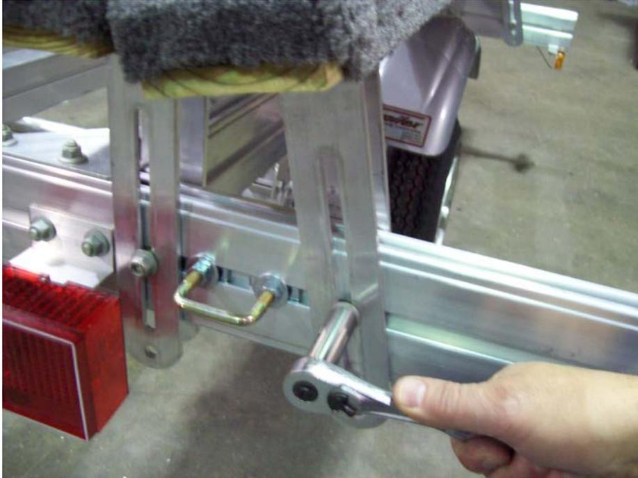
Install the outer cradle assembly, position and tighten nuts. Final adjustments will be made when the boat is fitted to the trailer.
