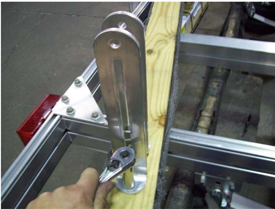
Install slotted brackets on the underside of the 6' padded cradle as shown. Reinstall nuts and lock washers, then tighten nuts. Repeat the process for the other cradles.
