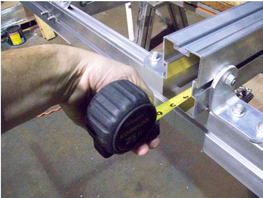
Extend a tape measure inside the tongue from the rear of the trailer until it protrudes at the front of the trailer under the coupler.
