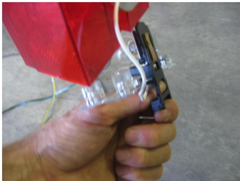
Locate the black tab at the bottom of the tail light. Move the tab toward the rear of the trailer and pull down releasing the bulb assembly from the light housing.
