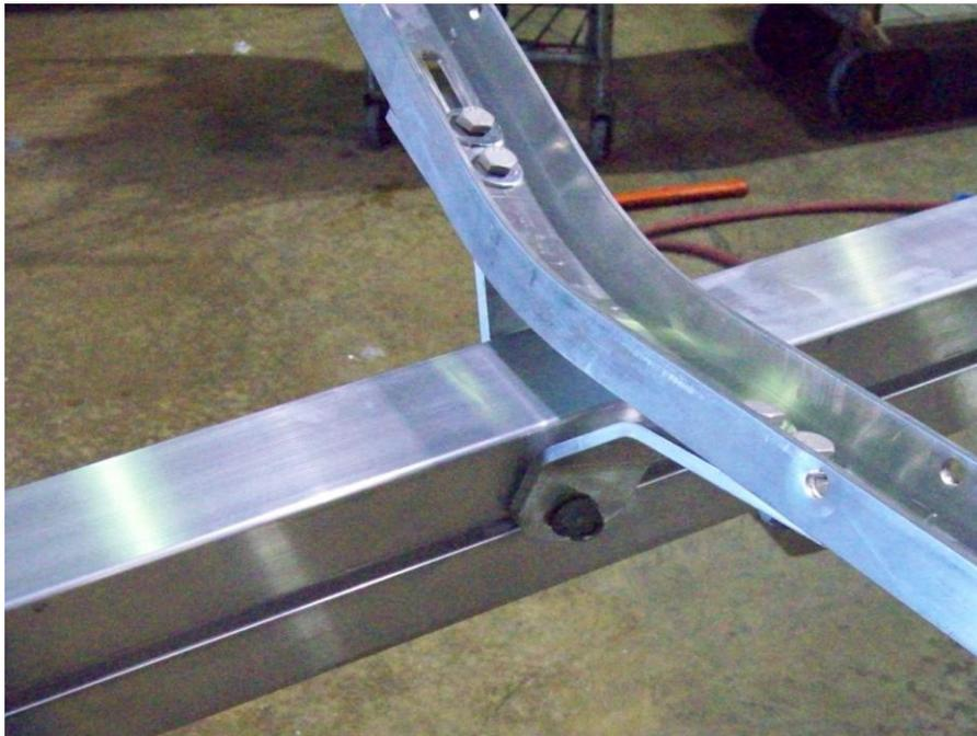
Position the rear cradle holder assembly about 12” from the rear and repeat the steps to install the padded cradles.
