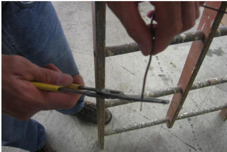
Cut the exposed strands of wire off of the end of the brown wire on the right (passenger side) running light.
