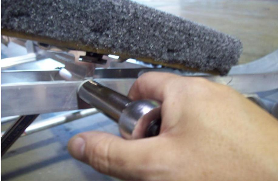
Install the padded cradle (inner position shown – this may vary depending on the width of the hull). Final angle will be determined when the trailer is fitted to the boat.
