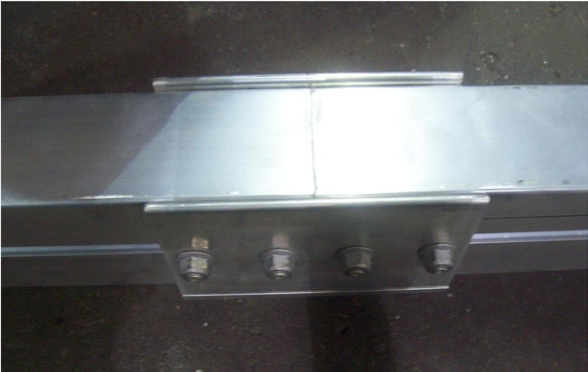
Tighten all 12 nuts making sure that the tongue sections are as tight as possible to one another. (top of tongue)
