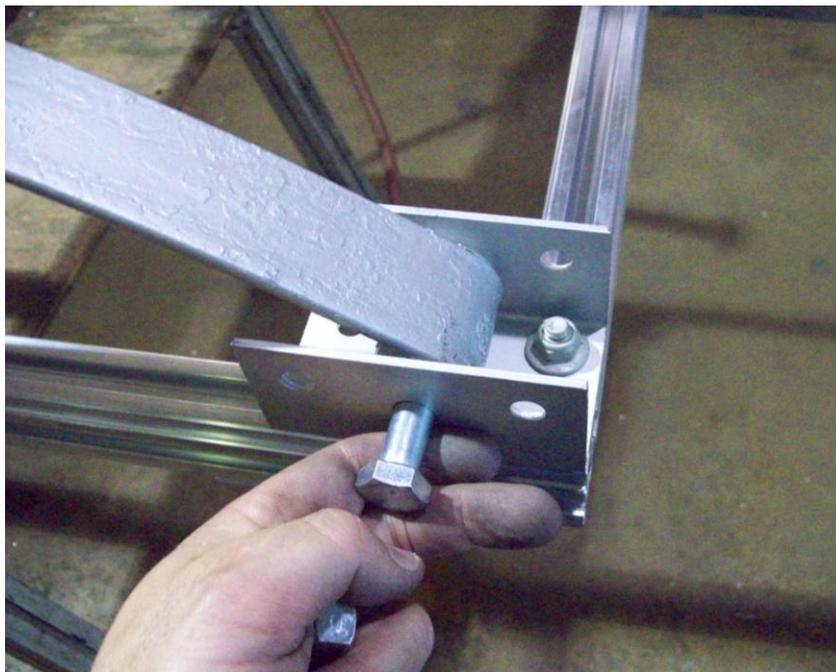
Remove the bolt from the front spring eye and install the spring into the spring hanger in the center hole with the nut towards the inside of the trailer. Do not tighten yet.
