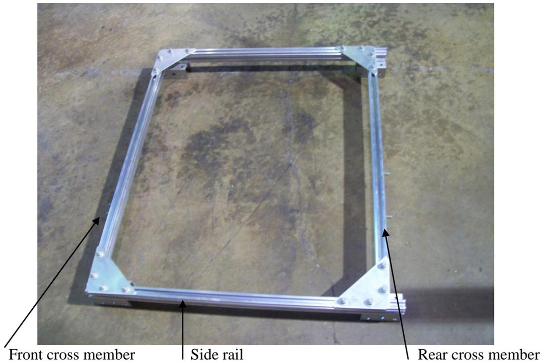
Next layout the front and rear cross member and slide the side rails through them to make a square frame as shown.
