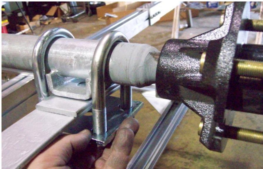
Locate the U-bolts and tie plates and install them as shown.
