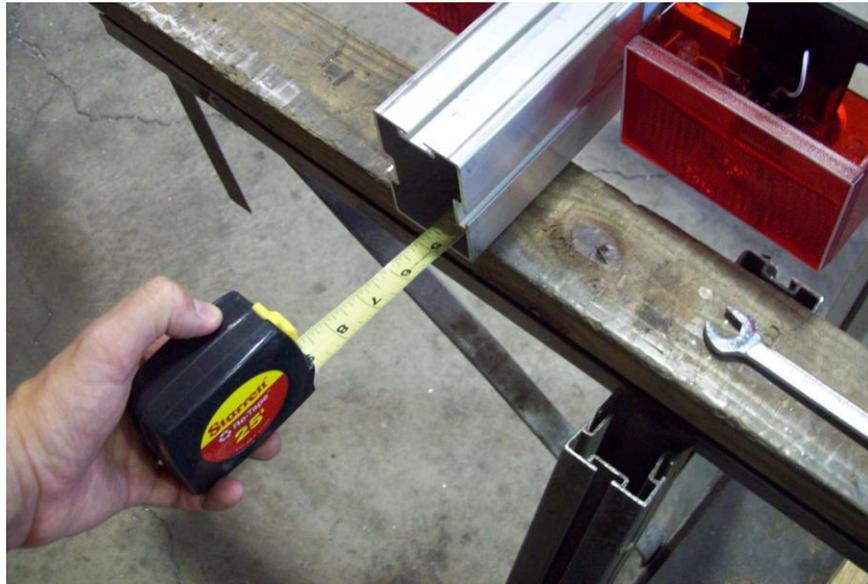
Extend a tape measure inside the tongue from the rear of the trailer until it protrudes at the front of the trailer under the coupler.
