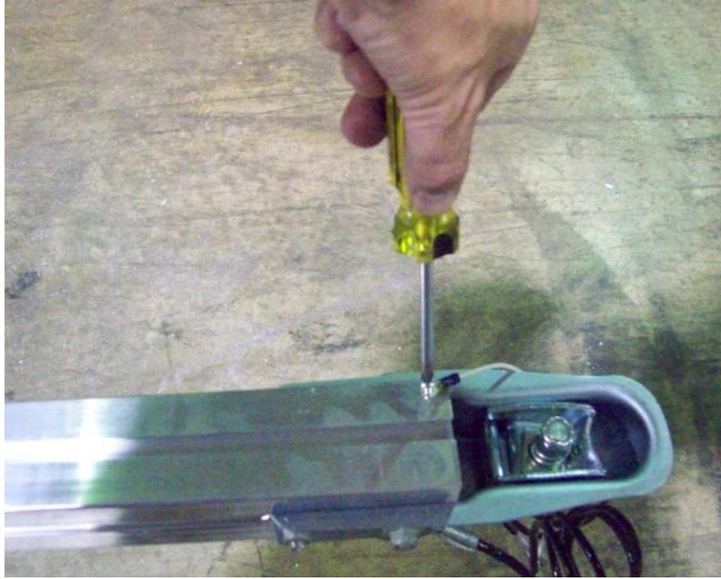
Install Philips screw through the ground wire into the pre-drilled hole located under the tongue just behind the coupler.
