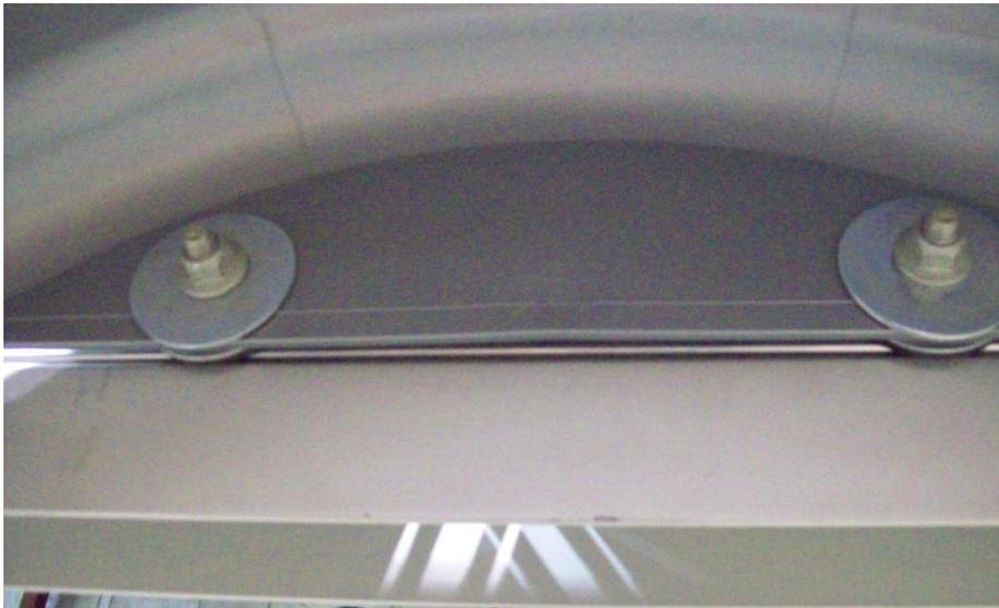
Install the fender, two more steel washers, and nuts, center the fender over the axle and tighten the nuts. Repeat for the other side.
