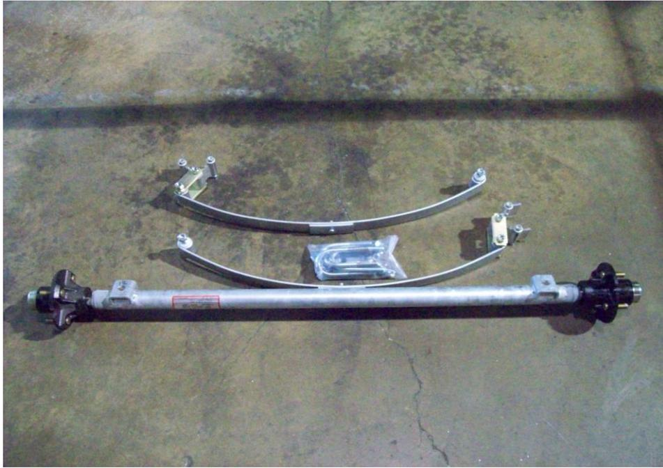
Axle assembly, springs and U bolt hardware.
