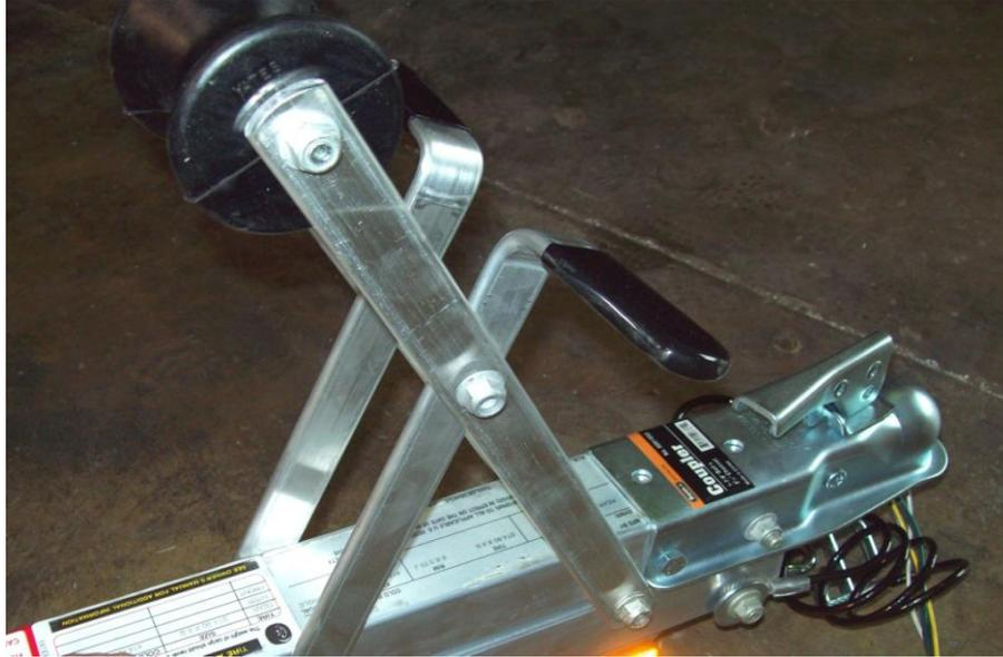
Using the 4 remaining T-bolts in the front tongue section, install the bow stand with the roll facing the rear of the trailer and the handles facing forward as shown.
