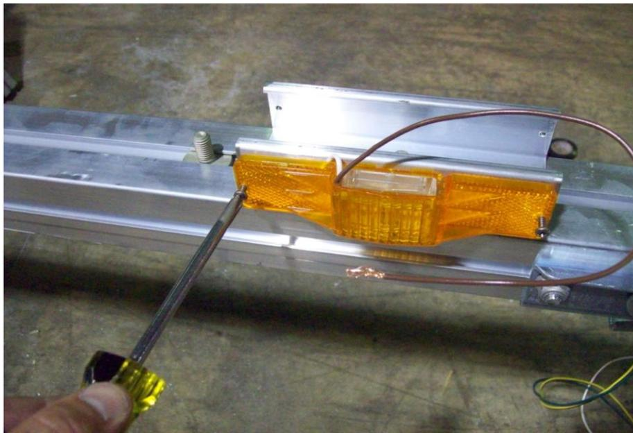
Install the running lights into the pre-drilled holes in the running light bracket using a Philips screwdriver. Be sure the screw is through the ring terminal on the back side of the lights. This will supply a ground to the lights. **DO NOT OVER TIGHTEN**
