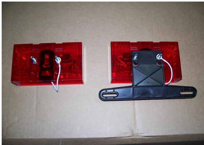
Mount the license plate bracket to the driver side tail light.
