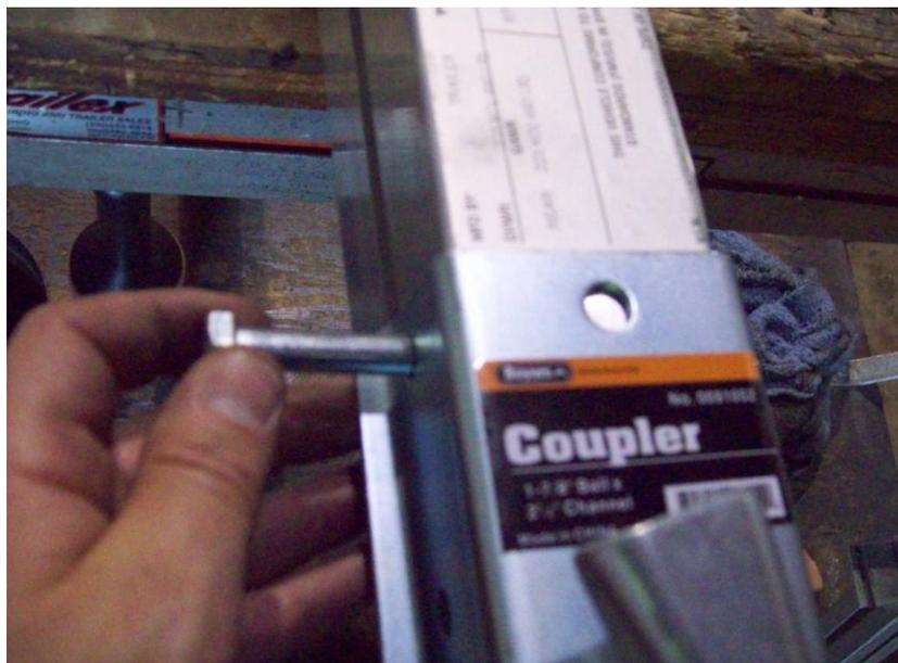
Install a 3 1/4" bolt through the rear hole of the coupler.
