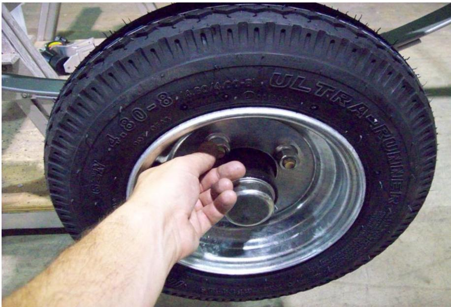
Install the wheels with the valve stems facing out. Install the lug nuts with the tapered side facing the wheel
