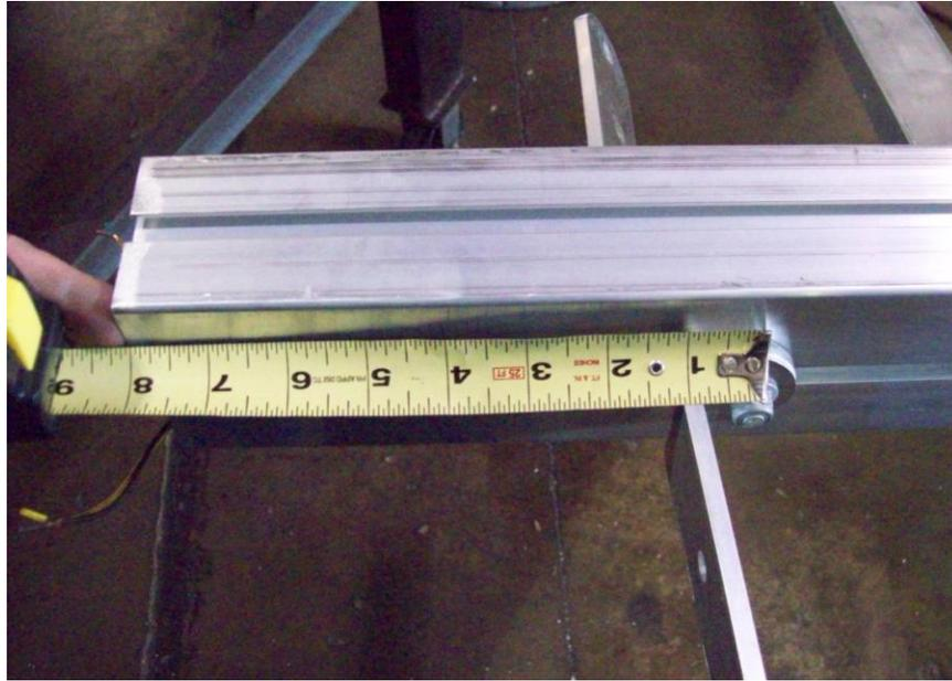
Install light bracket on both sides of the tongue section 8" from the back.
