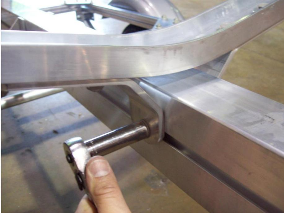
Tighten the nuts making sure the cradle holder brackets are perpendicular to the tongue.
