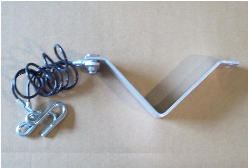
Skid and safety hitch cables.
