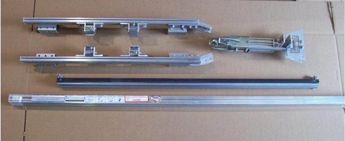
Side rails, rear cross member, diagonal rails, and tongue section with coupler.
