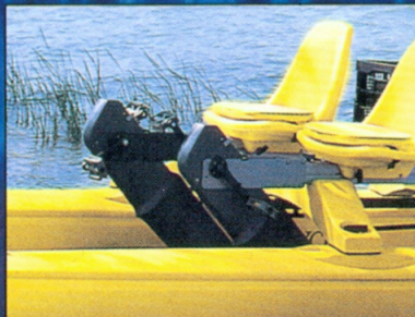
Rotating and removable drive kicks up automatically for landing
